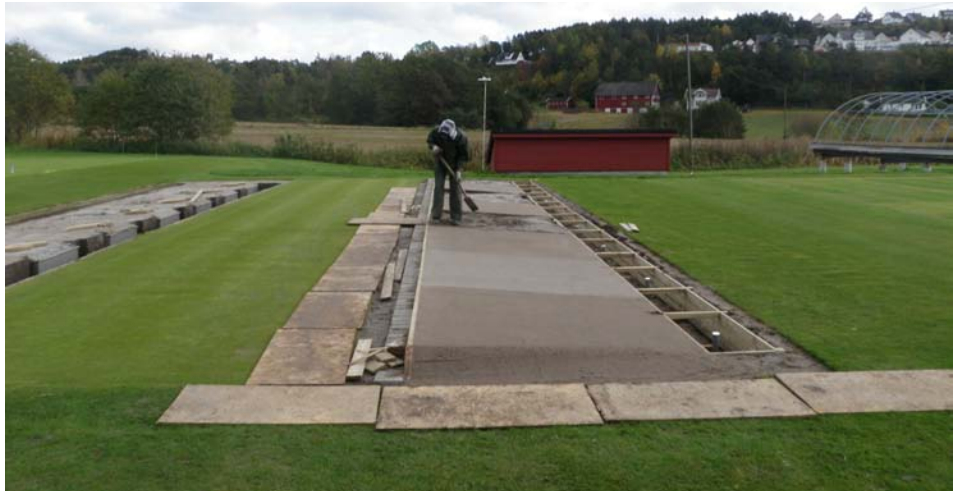
Photo 2. Preparing experimental greens before seeding or sodding in May 2016. Compost amended rootzones had darker color than peat-amended rootzones. All greens were prepared with a surface inclination of 5 % to the south, allowing surface water to be collected in containers in the trench to the right.
