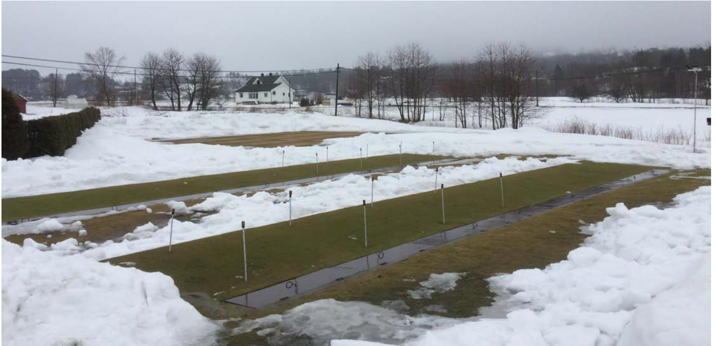
Photo 7: Experiment on 23 March 2018. Snow above ice cover had been removed three times during the winter.
