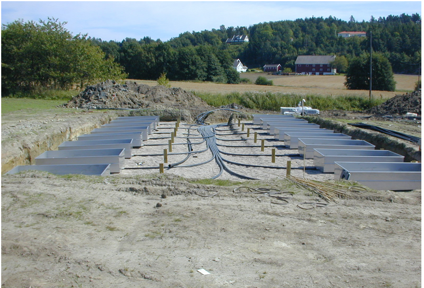
Photo 1. Lysimeters (1 m x 2 m) for collection of drainage water from experimental USGA-spec. greens at NIBIO Landvik, Norway
