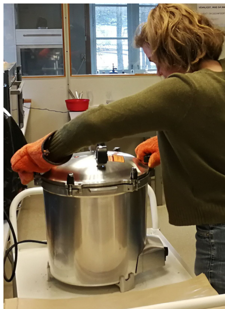
Photo 2. Kristine Sundsdal sterilises glass vials with growth medium by autoclaving and makes them ready for seeding, 15 Feb. 2019. Photo: T. Espevig.
