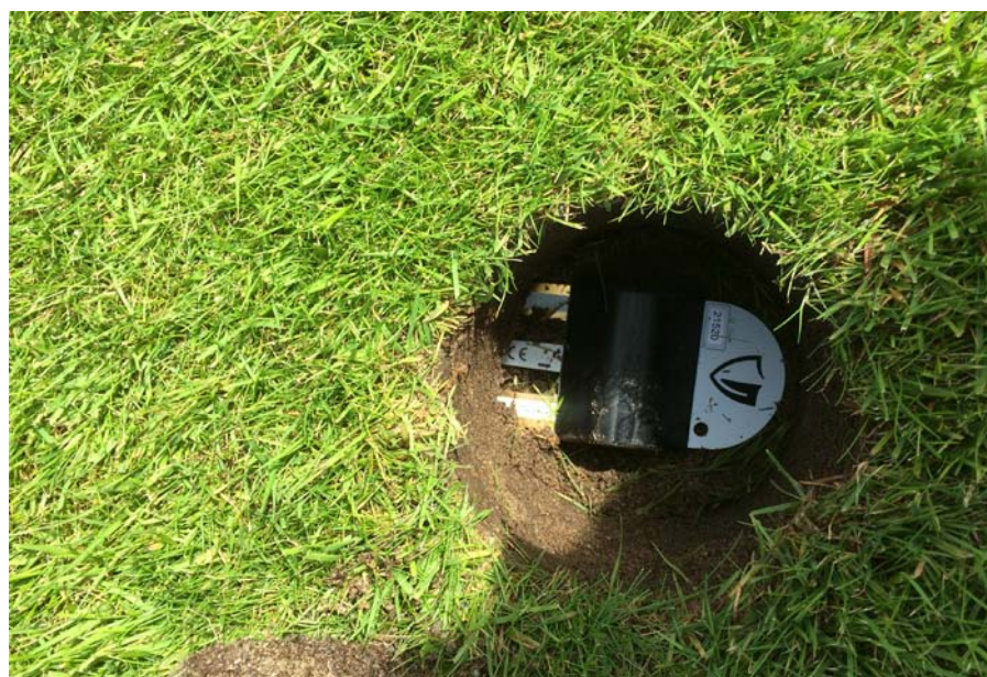
Photo 5a,b. Volumetric soil water content is measured continuously by remote sensors installed at 10 cm depth in each plot (left) and three times a week using a TDR instrument with 20 cm rods (right). The remote sensor units have been provided by the Norwegian technology company Agdir as an in-kind contribution to the project. Photo: Trygve S. Aamlid.
