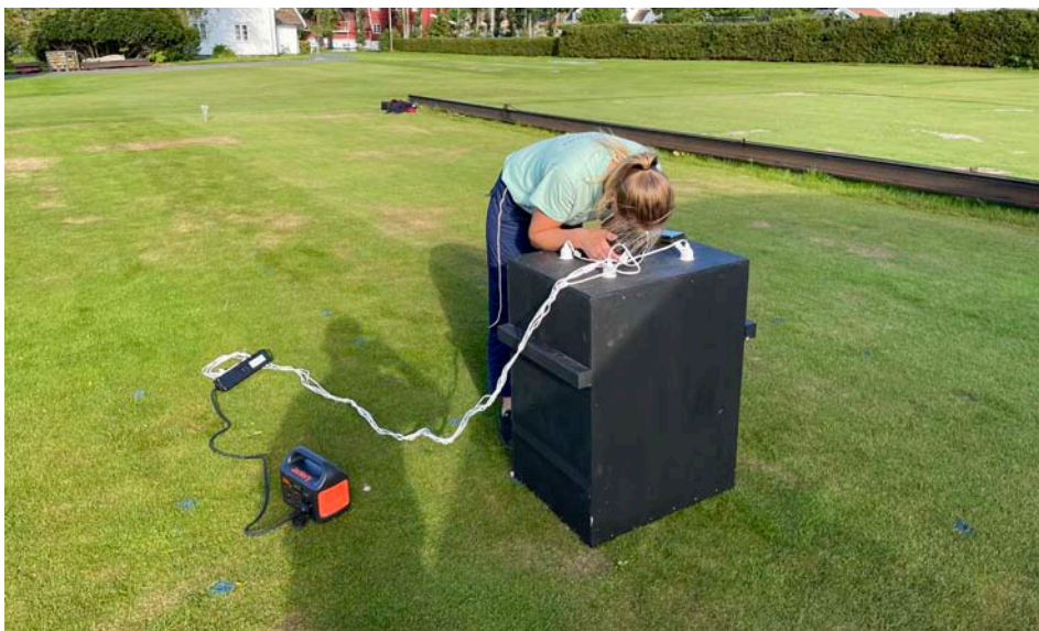
Photo 6. During the drought periods, digital images are taken three times a week to determine turfgrass green coverage. Photo: Trygve S. Aamlid
