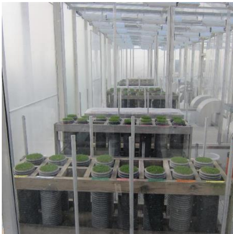
Phytotron compartments for WP 1 and 2 with temperatures: 7, 12 and 17 °C. Photo: Anne F. Øgaard
