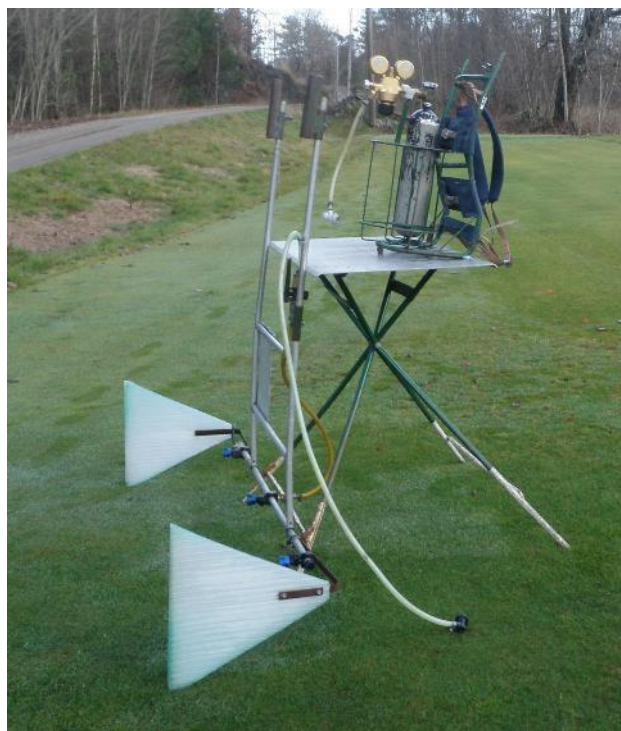
Photo 3. Experimental plot backpack sprayer used for application of Qualibra and Primo Maxx. Photo: Trygve S. Aamlid
