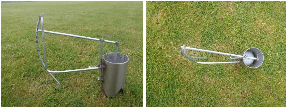
Photo 6a,b. Custom-made instrument used to determine golf ball lie on fairways. Photo: Trygve S. Aamlid
