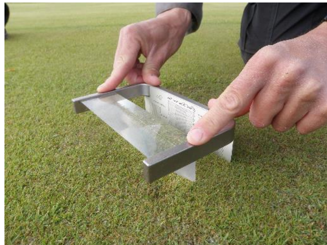
Photo 7. Prism used for accurate measurement of turfgrass height. Photo: Trygve S. Aamlid.
