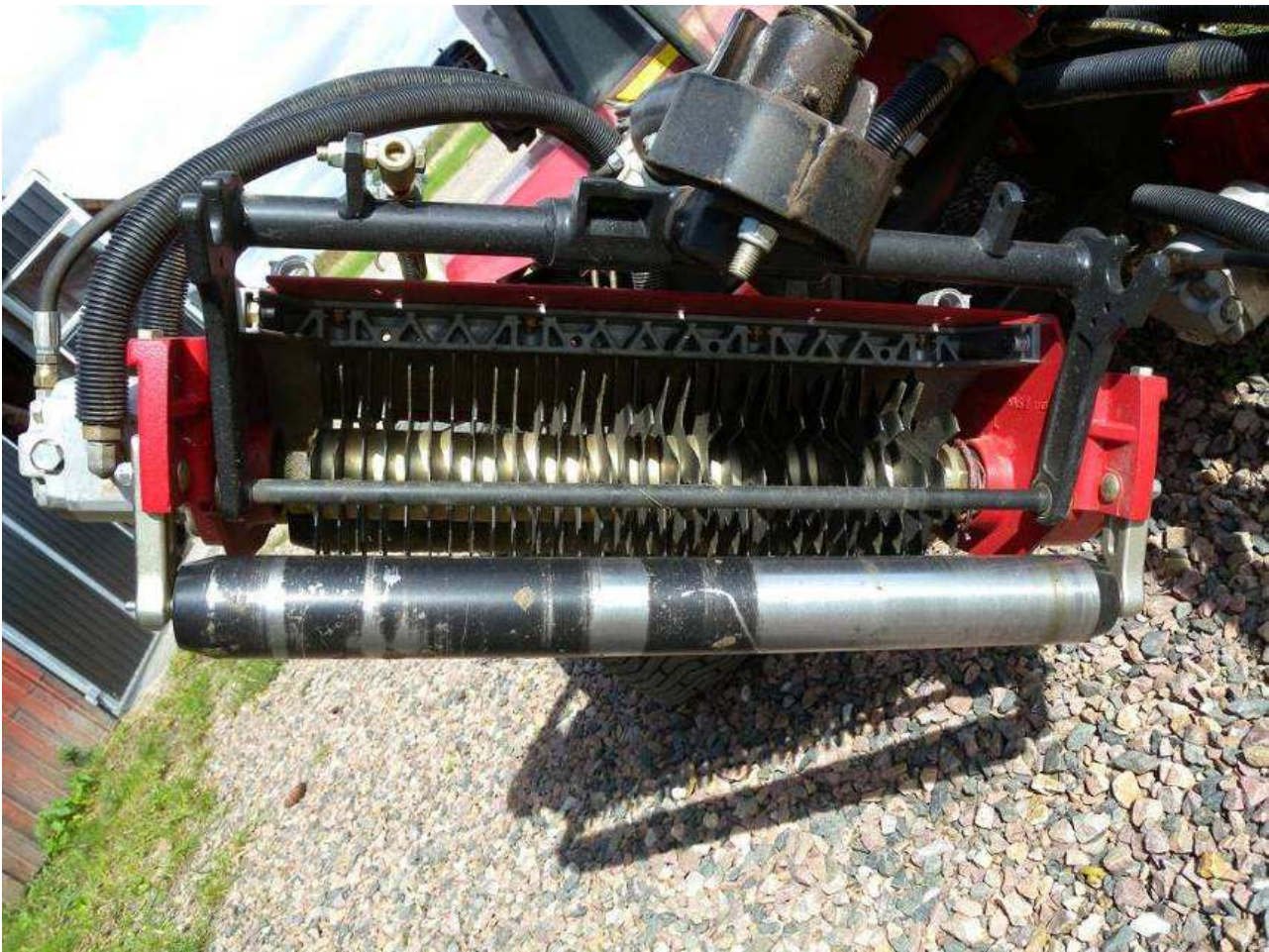
Picture 12. Vertical cutting equipment. Photo; Håkan Rasmusson.
