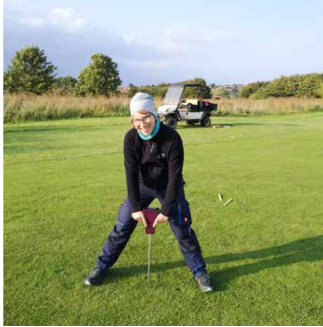
Photo 2. Measuring soil compaction.
