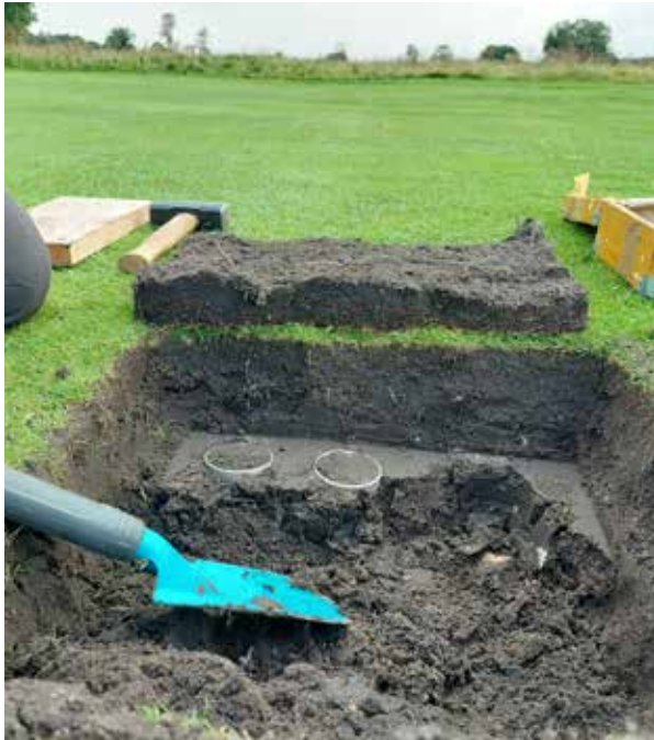
Photo 1. Undisturbed soil cylinders taken out.
