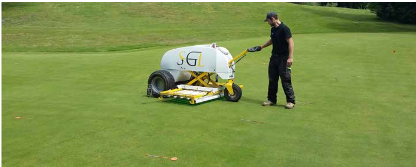
Photo 19. Application of UV-C radiation with SGL UVC 180 unit on the putting green of Osnabrück GC. Photo:Wolfgang Prämaßing.
