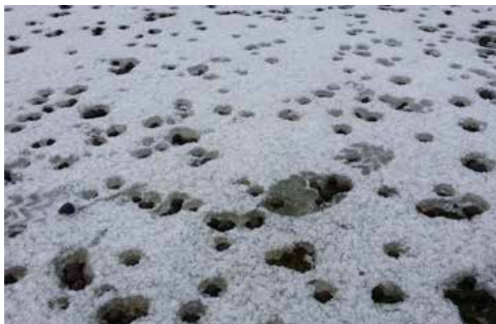
Photo 33a,b LECA® can be used to penetrate ice if there is some solar radiation. These photos are from Sunnfjord GC, Norway. The aggregates melted holes in the ice even though the weather was partly cloudy. Photo: Leiv Årseth.
