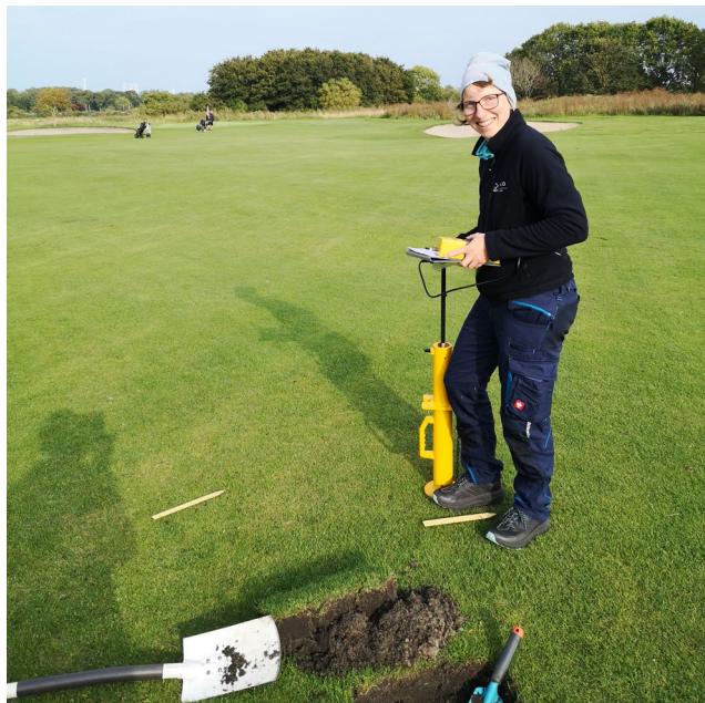
Photo 4. Measuring surface hardness with the Clegg Soil Impact Tester at Grenå GC (Photo: Karin J. Hesselstøe).
