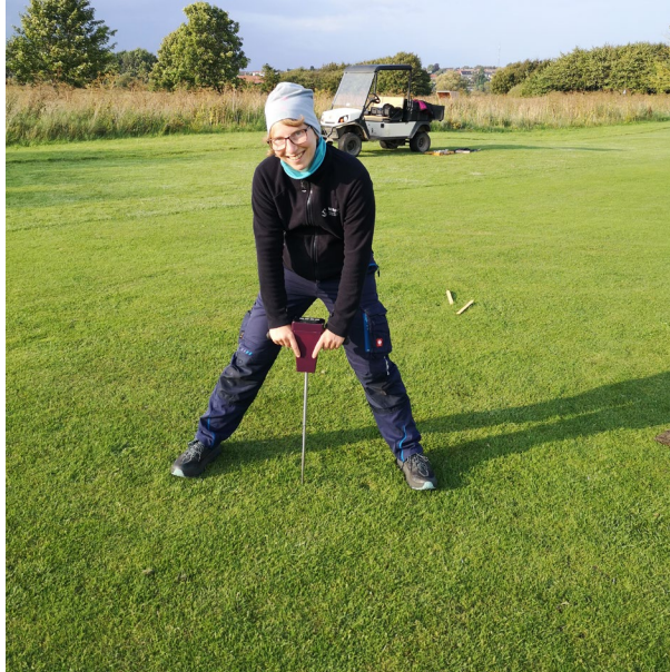
Photo 3. Penetrometer measurements using the Field Scout SC900 Soil Compaction Meter at Grenå GC (Photo: Karin J. Hesselstøe).
