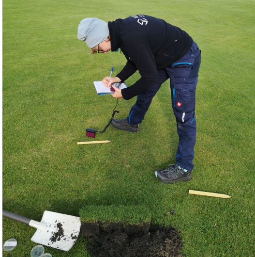
Photo 5. Soil water content measurements with Field Scout TDR 100 Soil Moisture Meter at Grenå GC (Photo: Karin J. Hesselstøe).
