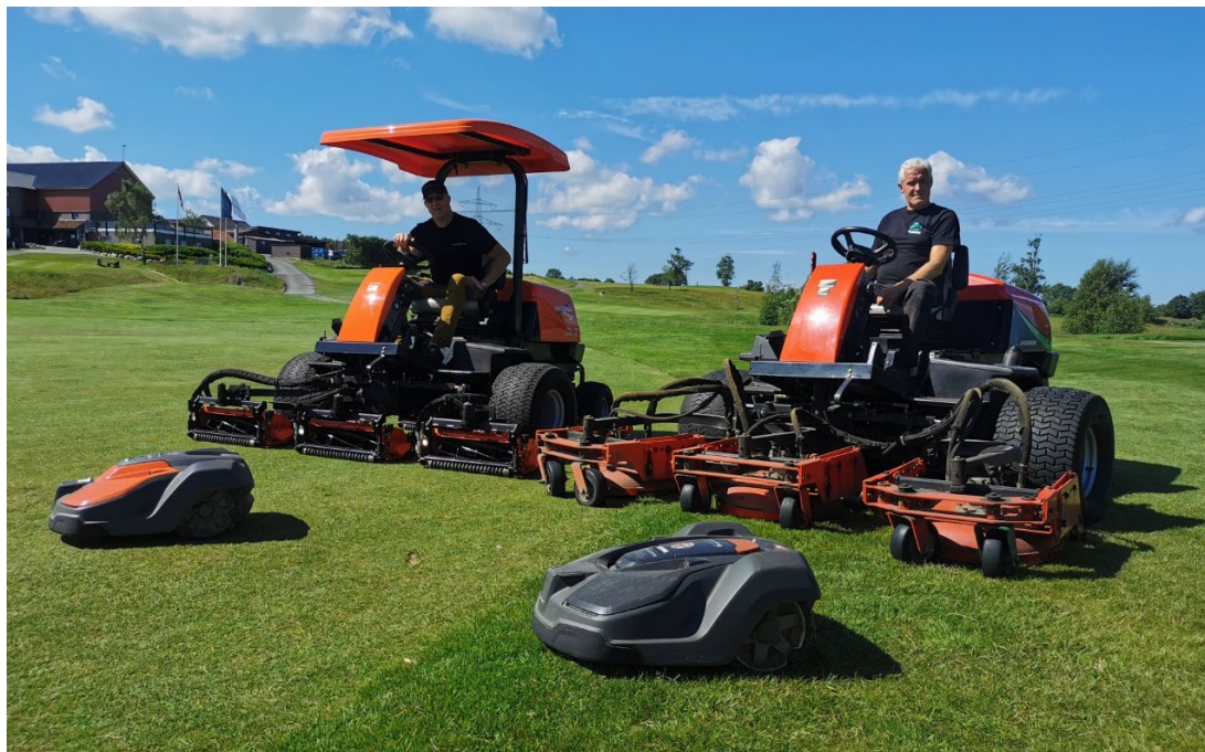
Photo 1. Traditional and robotic mowers at Sandnes GC. To the left traditional Jacobsen 250 reel mower and robotic Husqvarna 550. Photo: Sandnes GC.
