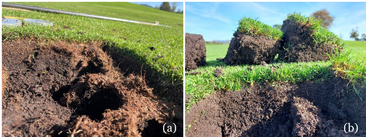
Photo 6. Soil profile at 0 – 20 cm depth on traditional mown fairway (a) and robotic mown fairway at Sandnes GC (b); Photos: Anne F. Borchert.
