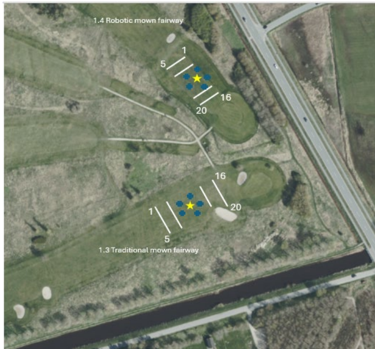
Figure 5. The 5 th and 8 th fairways with the location of the registration areas at Grenå Golf Club. The yellow stars indicate the location of the soil pit where samples for bulk density, porosity, field capacity, and grain size distribution were taken. The blue crosses indicate where soil water content, surface hardness, and penetrometer measurements were taken (n=5). The white lines show where additional penetrometer measurements were taken on four transects (n = 20; 5 measurements along each line; numbers = measurement ID). https://dataforsyningen.dk/map
