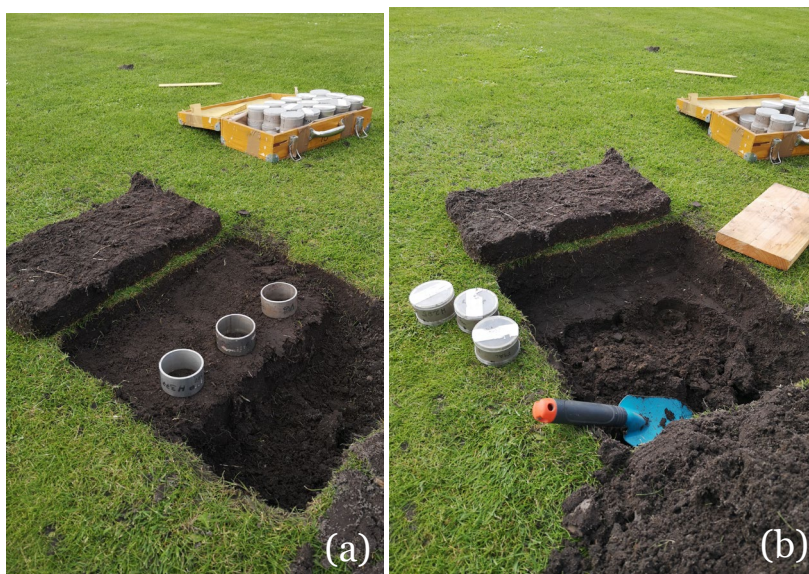
Photo 2. The soil corers were placed on the soil surface before forcing them into the soil (a) and removed afterwards using a small shovel (b). In the background, the wooden case for transportation is shown (Photos: Anne F. Borchert).
